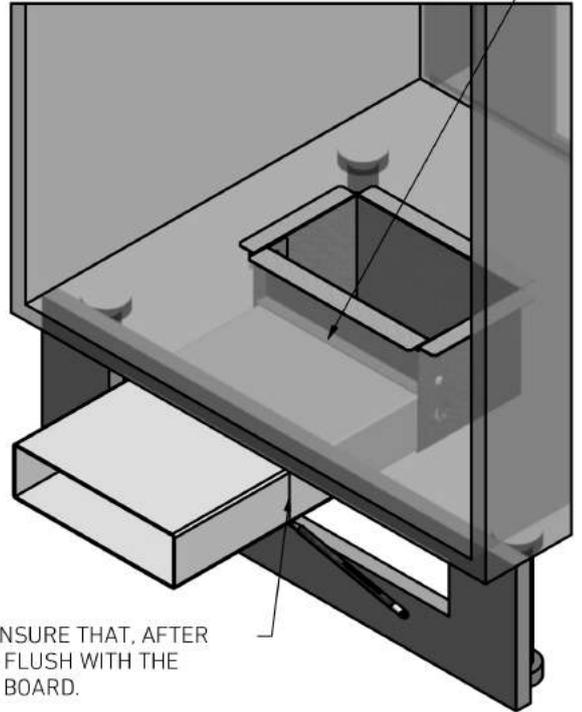
WHEN MARKING TO CUT ENSURE THAT, AFTER CUTTING, THE DUCTING IS FLUSH WITH THE FRONT FACE OF THE KICK BOARD.
