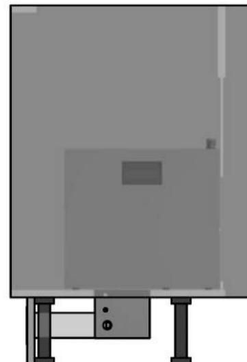
THE DRY039 CHILLER/CARBONATOR UNIT MUST BE PLACED TO THE LEFT AND REAR MOST POSITION INSIDE THE CABINET TO ENSURE THE VENTILATION OPENINGS ARE IN LINE WITH THE OPENINGS CUT INTO THE CABINET.
