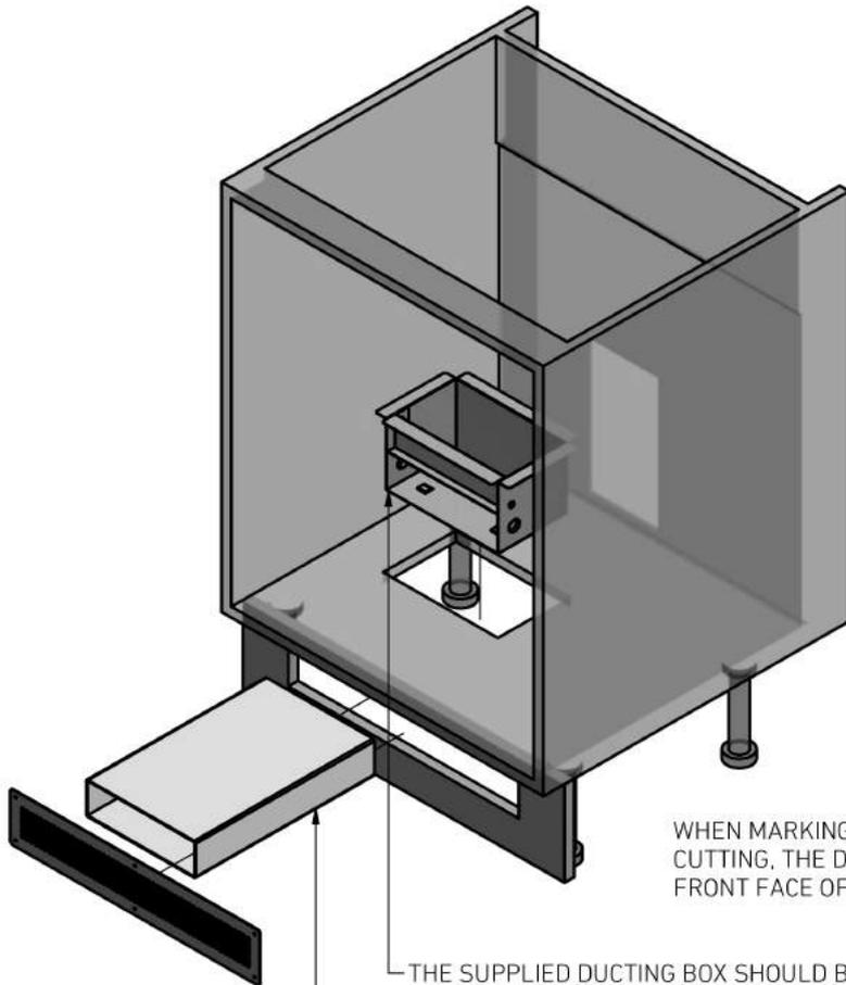
THE DUCTING SLOTS INTO THE OPENING OF THE DUCTING BOX. INSERT THE DUCTING UNTIL IT REACHES ITS LIMIT STOPS.
